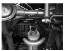
3. Slide muffler #B no less than  $1\frac{1}{2}$ " and no more than 2" onto the front headpipe with louvers in muffler facing towards the converter. Use a jack stand to support the muffler. Outlet of muffler should be clocked at 9 o'clock. Attach using clamp #G. Install rear hanger #F onto muffler. Do not tighten. Muffler inlet is looking into the louvers.
