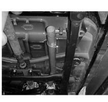
Bolt on front headpipe #A using bolt kit #I and gasket #H. Use a RTV gasket sealer for flange connection. (Note Headpipe will lean toward passenger side.)
