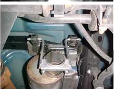
Install muffler #A onto factory headpipe with the flange end of the muffler using gasket #E and using bolt kit #F, Make sure the outlet of the muffler is at the 4 o'clock position.
