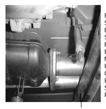
REMOVE O2 SENSOR FROM STOCK HEAD PIPE AND UN-BOLT STOCK HEAD-PIPE. STOCK NUTS AND BOLTS WILL BE RE-USED. CUT STOCK EXHAUST JUST BEHIND THE MUFFLER FOR EASIER REMOVAL. LEAVE ALL RUBBER GROMMETS IN PLACE. FOR EASIER REMOVAL OF HANGERS SPRAY WD-40 TO AID YOU IN REMOVING THEM.
