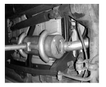
SLIDE MUFFLER #B WITH DUAL INLET ONTO HEADPIPE AT LEAST 1-1/2" TO 2". MUFFLER OUTLET SHOULD BE AT THE 12 O'CLOCK POSITION. USE CLAMPS #F TO ATTACH IT TO THE HEADPIPE. MAKE SURE INLETS AND MUFFLER IS LEVEL. USE JACK STAND TO SUPPORT MUFFLER. DO NOT TIGHTEN.
