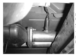
RE-INSTALL O2 SENSOR. USE A SMALL AMOUNT ANTI- SEIZE ON THE THREADS. NOW FIRMLY TIGHTEN ALL CLAMPS, HANGERS, FLANGE, AND BOLTS
