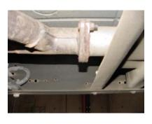
TO REMOVE STOCK EXHAUST UN-BOLT THE FACTORY FLANGE LOCATED IN FRONT OF THE MUFFLER. DO NOT THROW AWAY THE STOCK BOLTS AND NUTS. YOU WILL RE-USE THEM. LEAVE ALL RUBBER GROMMETS IN PLACE. USE WD-40 TO AID IN REMOVAL OF THE STOCK EXHAUST AND HANGERS.
