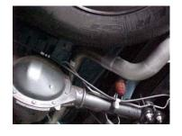
Insert welded hanger into rubber grommet.
