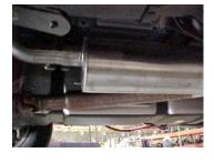
Install muffler onto head pipe 1-1/2" to 2" with the louvers facing towards the converter. Use a jack stand to support the muffler. Use clamp #F to secure the muffler to the head pipe. Do not tighten. Muffler inlet is looking into the louvers. Outlet should be at the 11 o'clock position.
