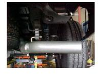
Install the turnout pipe #D on to the tailpipe. Secure together with clamp #F. Do not tighten. Roll the exit pipe until it is at the correct angle for your truck. Insert welded hanger into rubber grommet.
