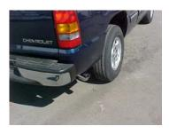
Install stainless steel tip. Clamp down. When you have everything in place, firmly tighten all bolts and clamp down securely. To clean stainless steel tip use any stainless steel cleaner and Scotch Brite pad.
