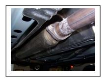
Lay out the exhaust on the floor so it looks like the drawing and compare parts with manual. To remove the stock exhaust Cut off your stock muffler, remove the of your stock exhaust from the 2-bolt flange located behind the factory catalitic converter.
