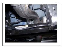
Install the over axle tailpipe # c onto the front pipe 1-1/2" to 2". Secure to the tailpipe using clamp # F. Do not tighten.
