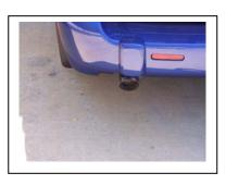
Install stainless steel tip. Clamp down. When you have everything in place, firmly tighten all bolts and clamps down securely. To clean stainless steel tip use any stainless steel cleaner and Scotch Brite pad.
