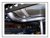
Install frontpipe # B 1-1/2" to 2" into the resonator. Use clamp # F to secure the tailpipe to the muffler. Do not tighten.
