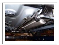
Install resonator # A on to your existing stock 2-bolt flange and secure with bolt kit # E. Use a jack stand to support the resonator.
