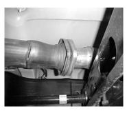
FOR AN EASIER REMOVAL OF THE FACTORY EXHAUST CUT THE TAILPIPE BEHIND THE REAR MUFFLER HANGER. THEN UNBOLT THE FLANGE BEHIND THE CONVERTER. **KEEP THE BOLTS FOR YOU WILL REUSE THEM.** USE WD-40 ON ALL HANGERS. LEAVE ALL FACTORY RUBBER GROMMETS IN PLACE.
