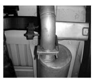
INSTALL MUFFLER WITH THE INSIDE LOUVERS FACING FORWARD TOWARDS THE CONVERTER. USE CLAMP #E AT THE INLET OF THE MUFFLER. DO NOT TIGHTEN. MUFFLER OUTLET WILL BE POSITIONED AT ABOUT 8 - 9 O'CLOCK. THE MUFFLER INLET IS LOOKING INTO THE LOUVERS.
