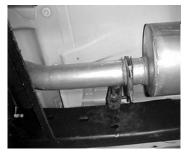
BOLT HEADPIPE #A RE-USING THE FACTORY NUTS. DO NOT TIGHTEN. INSTALL HANGER #G ONTO HEAD PIPE. SLIDE HANGER INTO RUBBER GROMMENT.
