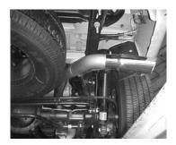
USE CLAMP #E TO SECURE THE PIPE TO THE MUFFLER. DO NOT TIGHTEN. INSERT WELDED HANGERS INTO RUBBER GROMMETS.
