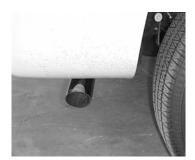
INSTALL THE STAINLESS STEEL TIP. USE ANY ALUMINUM OR STAINLESS CLEANER TO POLISH YOUR TIP.NOW, FIRMLY TIGHTEN ALL CLAMPS, HANGERS AND FLANGE.
