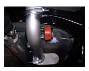
**5.** Install the intermediate tailpipe #C into the muffler  $1\frac{1}{2}$ "-2". Use clamp #G to secure tailpipe to muffler. DO NOT TIGHTEN.
