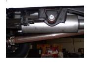
**4.** Slide muffler #B onto headpipe 1 ½"-2". Use jack stand to support muffler. Use clamp #F to secure muffler to headpipe. Next, install band clamp #G onto muffler. Insert hanger into rubber grommet. Use bolt kit #H to secure band clamp. Do not tighten.
