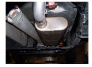
**4.** Install muffler onto head pipe #A. 1½"-2" with the louvers facing towards the converter. Use a jack stand to support the muffler. Use clamp #E to secure the muffler to the headpipe. DO NOT TIGHTEN. Muffler inlet is looking into the louvers. Outlet will be on the drivers side.
