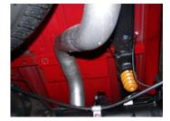
5. Install the over axle tailpipe #C onto the outlet of the muffler 1.5"-2" using clamp #E to secure pipe to muffler.
