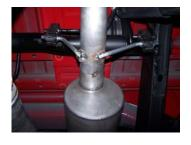
4. Slide the muffler into the headpipe at least 1.5"-2". Use a jack stand to support the muffler. Use clamp #E to secure muffler assembly to the headpipe. The outlet of the muffler will be at approximately 11 o'clock. The muffler inlet is looking into the louvers. Do not tighten.
