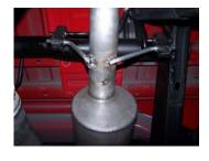
4. Slide the muffler into the headpipe at least 1.5"-2". Use a jack stand to support the muffler. Use clamp #E to secure muffler assembly to the headpipe. The outlet of the muffler will be at approximately 11 o'clock. The muffler inlet is looking into the louvers. Do not tighten.
