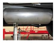
4. Install muffler #B onto head pipe 1½"-2" with the louvers facing towards the converter. Use a jack stand to support the muffler. Use clamp #F to secure the muffler to the headpipe. DO NOT TIGHTEN. Muffler inlet is looking into louvers.
