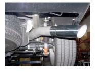
7. Install exit pipe #D into the tailpipe 1½-2" and secure with clamp #F. DO NOT TIGHTEN. Rotate pipe to best suit your vehicle.
