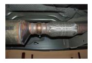
2. Remove the stock exhaust by unbolting it at the flange located in front of the muffler. Disengage the welded hangers from the OEM rubber grommets. Use WD-40 to aid in this process. Do not damage stock nuts and bolts or remove the rubber grommets as you will re-use them to mount your new system. Now, cut off tailpipe and remove system.
