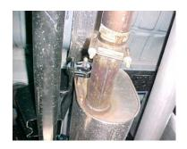
LAY OUT THE EXHAUST ON THE FLOOR SO IT LOOKS LIKE THE DRAWING AND COMPARE PARTS TO THE MANUAL. YOU MAY NEED TO HEAT IT UP FOR EASIER REMOVAL. LEAVE ALL RUBBER GROMMETS IN PLACE.
