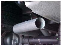
INSTALL EXIT PIPE #D OVERAXLE PIPE. ROLL TURNOUT PIPE UNTIL YOU HAVE IT AT THE CORRECT ANGLE FOR YOUR TRUCK AND CONNECT WITH CLAMP # F. BUT DO NOT TIGHTEN.
