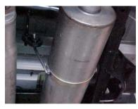
SLIDE BAND CLAMP #H ONTO MUFFLER #B. INSERT HANGERS INTO RUBBER GROMMETS AND ATTACH WITH #I.
