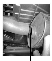
DO NOT REMOVE THE STOCK HEADPIPE.CUT 1 ½" IN FRONT OF STOCK MUFFLER.
