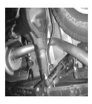
INSTALL THE OVERAXLE TAILPIPE #B INTO THE REAR OF THE MUFFLER 1 ½" TO 2". INSERT WELDED HANGER INTO RUBBER GROMMET. USE HANGER #D TO ATTACH THE OVERAXLE PIPE TO THE MUFFLER. DO NOT TIGHTEN. SPARE TIRE MAY NEED TO BE LOOSENED AND PUSHED TO THE DRIVER SIDE FOR CLEARANCE PURPOSES.
