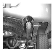
ADJUST THE OVERAXLE TAILPIPE UNTIL YOU HAVE A MINIMUM OF A 1" CLEARANCE AWAY FROM ALL PIPES, ETC. EXHAUST WILL EXIT STRAIGHT OUT THE REAR ON THE PASSENGER SIDE.
