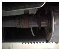
Lay out the exhaust on the floor so it looks like the drawing and compare parts with manual. To remove the stock exhaust remove it from the clamp in front of the muffler, remove ground strap, do not disguard hardware you will re-use it. You may need to heat it up for easier removal. Leave all rubber grommets in place. Use WD-40 to aid in removal of exhaust and hangers.
