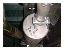
Install muffler # B onto head pipe 1-1/2" to 2" with the louvers facing towards the converter. Use a jack stand to support the muffler. Use a jack stand to support the muffler. Use clamp # E to secure the muffler to the head pipe. Do not tighten. Muffler inlet is looking into the louvers. Outlet should be at the 1 O'clock position.
