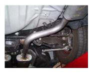
Now go back and make sure the first two mufflers in the middle are level. Then push up on factory cross member before tightening clamps. Then tighten Xpipe. Next, with both tailpipes in place tighten all bolts and clamps securely.
