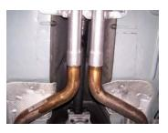
Lay out the exhaust on the floor so it looks like the drawing and compare parts with manual. To remove the stock exhaust, first you must remove the factory cross member under the X-pipe. Then unbolt and remove driver side tailpipe at the flange. Now unbolt and cut tack welds on factory clamps at the X-pipe and carefully remove factory exhaust, save clamps for new exhaust installation. Leave all rubber grommets on hangers. Use WD-40 to help remove hangers.
