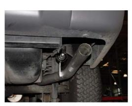
INSTALL OVERAXLE TAILPIPE #B INTO **MUFFLER 1-1/2**" TO 2". INSERT WELDED HANGER INTO RUBBER GROMMET, IF YOU REMOVED REAR HANGER BRACKET **RE-INSTALL IT** NOW. USE CLAMP #E TO SECURE TAILPIPE TO MUFFLER. DO NOT TIGHTEN.
