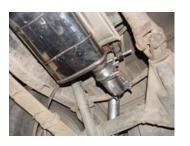
Next install front tailpipe #B into muffler 1  $\frac{1}{2}$  to 2". The shorter side goes into the muffler. Use clamp # F to secure pipe to muffler. Slide welded hangers into rubber grommets.
