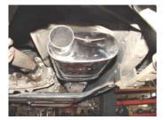
Install muffler # A Onto stock pipe, line up the notch. Use clamp #D to secure muffler to pipe. Do not tighten. Use a jack stand to support the converter.
