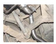
Next install over axle tailpipe #C onto pipe #B. Install hanger # F and slide hanger into rubber grommet. Use clamp #E to secure pipes together. Do not tighten. After checking for your proper clearness tighten all clamps starting from the front and working your way to the back.
