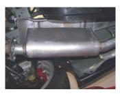
**2.** Unbolt factory muffler from flange located in front of muffler and remove. Repeat for other side.
