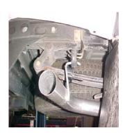
INSTALL WELDED HANGER INTO GROMMET.
