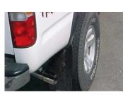
INSTALL THE STAINLESS TIP. USE A STAINLESS STEEL OR ALUMINUM CLEANER AND ANY SCOTCH BRITE PAD TO CLEAN. NOW TIGHTEN ALL HANGERS AND
