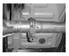
REMOVE STOCK EXHAUST BY UN-CLAMPING THE STOCK CLAMP AT THE HEADPIPE. BE CAREFUL NOT TO DAMAGE THIS CLAMP BECAUSE YOU NEED TO RE-USE IT. ONCE IT IS UN-CLAMPED, YOU WILL BE ABLE TO PULL THE STOCK EXHAUST OFF THE VEHICLE. MAKE SURE ALL FACTORY RUBBER GROMMETS ARE STILL IN FACTORY LOCATION. USE WD-40 TO AID YOU IN **REMOVAL OF THE HANGERS** FROM THE GROMMETS.
