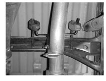
INSTALL HANGER #DINTO THE REAR MUFFLER RUBBER GROMMETS. THE VERTICAL RODS WILL BE FACING TOWARDS THE REAR OF THE TRUCK.
