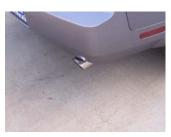
**4.** Install stainless steel tips. Clamp down. When you have everything in place, firmly tighten all bolts and clamps down securely. Use stainless steel cleaner and a Scotch Brite pad weekly to prevent tip from discoloration.
