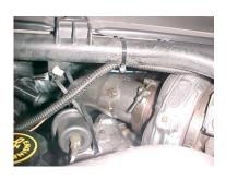
REMOVE THE REMAINING STOCK DOWN PIPE BY UNCLAMPING IT FROM THE TURBO HOUSING. USE A 11MM SOCKET OR WRENCH TO REMOVE YOUR STOCK PIPE THROUGH THE BOTTOM. DO NOT DISGARD THE STOCK CLAMP YOU WILL NEED TO RE-USE IT.
