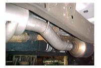
**3.** Install head pipe # A on to your existing stock front pipe and line up the notch. Then secure with clamp # H. Insert hangers into rubber grommets. Do not tighten.
