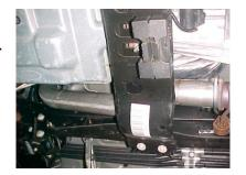
INSTALL PIPE #J ONTO PIPE #K. USE CLAMP #H TO SECURE PIPES TOGETHER. DO NOT TIGHTEN.
