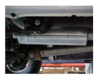
**5.** Install muffler # B onto head pipe # A 1-1/2" to 2" with the louvers facing towards the converter. Use a jack stand to support the muffler. Use clamp # G to secure the muffler to the head pipe. Do not tighten. Muffler inlet is looking into the louvers.
