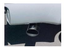
**9.** Install stainless steel tip. Clamp down. When you have everything in place, firmly tighten all bolts and clamp down securely. To clean stainless steel tip use any stainless steel cleaner and
