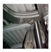
**7.** Next, remove spare tire. On pass. side there is a bracket that holds the spare tire in place. Remove it and spin it around 180 degrees. Now re-install your spare tire.
