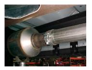
**2.** To remove the stock exhaust remove it from the clamp located just behind the catalytic converter. Cut off your stock tailpipe for easier removal. Leave all rubber grommets in place. Use WD-40 to aid in removal of exhaust and hangers.
