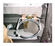
**4.** Install band clamp #F into rubber grommets located just above the axle. Do not tighten. And attach with bolt kit # I.
