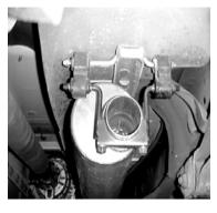
ONCE THE MUFFLER AND HEADPIPE ARE INSTALLED ROTATE THE MUFFLER AND HEADPIPE UNTIL MUFFLER OUTLET IS POSITIONED AT 3 O'CLOCK AND SITTING LEVEL UNDERNEATH THE VEHICLE. INSTALL THE O.E. HANGER #E ONTO OUTLET OF MUFFLER AND INSERT WELDED HANGERS INTO RUBBER GROMMET.
