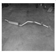
LAY OUT THE GIBSON EXHAUST AND COMPARE PART NUMBERS TO THE MANUAL. FOR AN EASIER REMOVAL LUBE ALL RUBBER GROMMETS WITH WD-40 AND CUT THE TAILPIPE DIRECTLY BEHIND THE MUFFLER. UN-BOLT THE FLANGE LOCATED IN FRONT OF STOCK MUFFLER. THEN REMOVE LEAVING ALL RUBBER GROMMETS IN PLACE. YOU WILL REUSE STOCK HEADPIPE FLANGE BOLTS.
