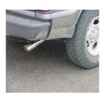
INSTALL YOUR STAINLESS STEEL TIP. USE ANY ALUMINUM OR STAINLESS STEEL CLEANER TO POLISH YOUR TIP. TIGHTEN ALL CLAMPS AND HANGERS. REINSTALL THE REAR SHOCK MOUNT.
