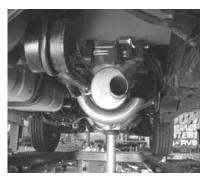
SLIDE MUFFLER #B ONTO HEADPIPE 1 1/2" TO 2". USE CLAMP #E TO SECURE MUFFLER TO HEADPIPE. DO NOT TIGHTEN. OUTLET SHOULD BE AT THE 3 O'CLOCK POSITION. MUFFLER INLET IS LOOKING INTO LOUVERS.
