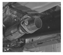
INSTALL FLANGE #G ONTO HEADPIPE #A. ATTACH TO FACORY FLANGE RE-USEING FACTORY BOLTS TO INSTALL IT. SNUG UP THESE BOLTS.
