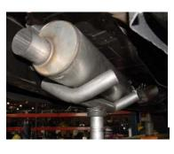
INSTALL MUFFLER #C ONTO TAILPIPE 1-1/2" TO 2" WITH INLET TOWARDS THE MOTOR. USE CLAMP #G TO SECURE THE TAILPIPE AND THE MUFFLER, DO NOT TIGHTEN. MUFFLER INLET SHOULD BE AT 9 O'CLOCK POSITION.
