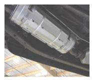
TO REMOVE STOCK EXHAUST UNBOLT IT FROM THE SLIP-FIT JOINT LOCATED IN THE REAR ABOVE THE AXLE AND SLIDE THE TAILPIPE OUT. NEXT UNBOLT THE 2-BOLT FLANGE LOCATED JUST BEHIND THE CATALYTIC CONVERTER. DO NOT THROW **AWAY STOCK NUTS AND BOLTS YOU WILL NEED TO RE-USE THEM.** NOW CUT OFF YOUR STOCK TAILPIPE JUST BEHIND THE MUFFLER AND REMOVE. LEAVE ALL RUBBER GEOMMETS ON THE HANGER. USE WD-40 TO AID IN THE REMOVAL OF EXHAUST AND HANGERS.
