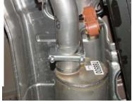
SLIDE FLANGE #A OVER GIBSON HEADPIPE #B. SLIDE HEADPIPE INTO MUFFLER 1-1/2" TO 2" USE CLAMP #H TO SECURE HEADPIPE TO MUFFLER. DO NOT TIGHTEN. NEXT USE YOUR STOCK NUTS AND BOLTS TO SECURE HEADPIPE TO STOCK FLANGE.
