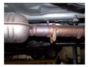
1. To remove the stock exhaust remove it from clamp located in front of the stock muffler. Disengage the welded hangers using WD-40 from the OEM rubber grommets. Do not damage or remove the rubber grommets as you will re-use them to mount your new system. Now, un-bolt tailbipe and remove exhaust.
