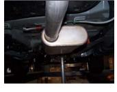
**3.** Install muffler #B onto head pipe  $1\frac{1}{2}$ "-2" with the louvers facing towards the converter. Use a jack stand to support the muffler. Use clamp #F to secure the muffler to the headpipe. DO NOT TIGHTEN.
