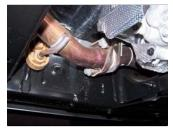
1. To remove the stock exhaust remove it from the 2-bolt flange located in front of the stock muffler. Disengage the welded hangers using WD-40 from the OEM rubber grommets. Do not discard, damage stock bolts or remove the rubber grommets as you will re-use them to mount your new system. Now, cut off tailpipe and remove exhaust.
