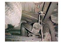
INSTALL TAILPIPE #C INTO MUFFLER 1 ½" TO 2". INSERT WELDED HANGER INTO RUBBER GROMMET. YOU WILL USE CLAMP #H TO SECURE PIPE TO MUFFLER. DO NOT TIGHTEN.
