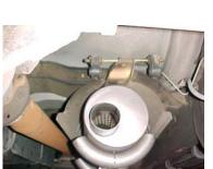
INSTALL MUFFLER #B 1 ½" TO 2" ONTO HEADPIPE WITH INLET TOWARDS THE MUFFLER. ROTATE MUFFLER UNTIL OUTLET IS AT THE 7 O'CLOCK POSTION. USE CLAMP #F TO SECURE. DO NOT TIGHTEN. NEXT, INSTALL REAR MUFFLER HANGER #H ONTO OUTLET OF MUFFLER. INSERT HANGERS INTO GROMMETS. DO NOT TIGHTEN. MUFFLER INLET IS LOOKING INTO THE LOUVERS.
