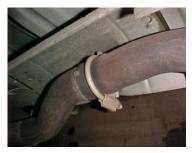
LAY OUT THE GIBSON EXHAUST ON THE FLOOR SO IT LOOKS LIKE THE DRAWING. TO REMOVE YOUR FACTORY EXHAUST REMOVE IT FROM THE CLAMP LOCATED IN FRONT OF THE MUFFLER. YOU MAY NEED TO HEAT IT UP FOR EASIER REMOVAL. USE WD-40 TO AID YOU IN REMOVING HANGERS LEAVE ALL RUBBER GROMMETS IN
