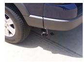
**6.** Install stainless steel tip #E. Clamp down. When you have everything in place, firmly tighten all bolts and clamps down securely. Use stainless steel cleaner and a Scotch Brite pad weekly to prevent tip from discoloration.
