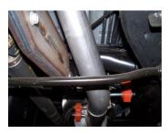
7. Install the over axle tailpipe #D into the extension pipe 1½-2". Use clamp #F to secure. Do not tighten. Insert welded hanger into the rubber grommet.
