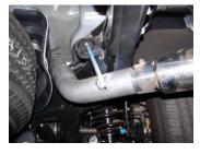
**8.** Install the exit pipe #E on the tailpipe. Secure together with clamp #F. Do not tighten. Roll the exit pipe until it is at the correct angle for your truck. Insert the welded hanger into rubber grommet.
