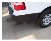
**11.** Install stainless steel tip. Clamp down. When you have everything in place, firmly tighten all bolts and clamps down securely. Use stainless steel cleaner and a Scotch Brite pad weekly to prevent tip from discoloration. Inspect all fasteners after 25-50 miles of operation and re-tighten as necessary
