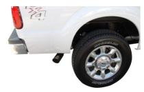
GIBSON EXHAUST systems are designed on a factory stock vehicle. Any aftermarket products installed could increase the sound levels of this Exhaust. Make sure there is a 1" clearance from ALL rubber brake lines, shock boots, fuel lines, tires, etc to prevent heat related damage.
