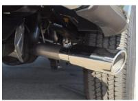
5. NOW INSTALL YOUR STAINLESS STEEL TIP. USE ANY ALUMINUM OR STAINLESS CLEANER TO POLISH YOUR TIP. THEN TIGHTEN ALL CLAMPS AND HANGERS.
