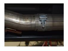
1. LAY OUT THE EXHAUST SYSTEM SO IT MATCHES THE DRAWING. MAKE SURE ALL PART NUMBERS ARE CORRECT. FOR AN EASIER REMOVAL OF THE FACTORY EXHAUST. CUT THE TAILPIPE JUST BEHIND THE FACTORY MUFFLER. LEAVE ALL RUBBER GROMMETS IN PLACE, USE WD-40 FOR EASIER REMOVAL OF FACTORY HANGER. UN **BOLT THE FACTORY CLAMP** LOCATED BEHIND THE FRONT RESONATOR AND REMOVE MUFFLER AND EXTENSION PIPE.
