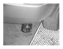
INSTALL YOUR STAINLESS STEEL TIP. USE ANY ALUMINUM OR STAINLESS STEEL CLEANER TO POLISH YOUR TIP. TIGHTEN ALL CLAMPS AND HANGERS.
