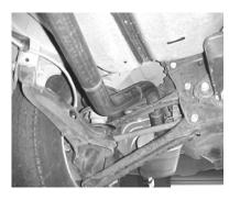
INSTALL REAR EXTENSION PIPE # B, USING CLAMP # F TO ATTACH TO RESONATOR.
