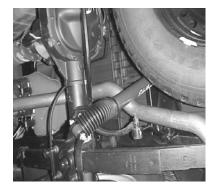
INSERT WELDED HANGER INTO THE RUBBER GROMMET.
