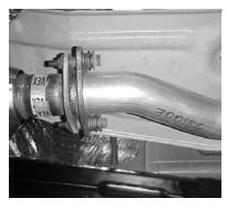
LAY OUT THE GIBSON EXHAUST SO IT LOOKS LIKE THE PICTURE AND COMPARE THE PART NUMBERS TO THE MANUAL TO MAKE SURE YOU HAVE THE CORRECT PART NUMBERS. THEN REMOVE THE FACTORY EXHAUST. FOR AN EASIER REMOVAL OF THE EXHAUST CUT JUST BEHIND THE MUFFLER ON THE TAIL PIPE. THEN UN-BOLT THE FACTORY FLANGE IN FRONT OF THE STOCK MUFFLER **NOTE**: **LEAVE ALL RUBBER GROMMETS IN PLACE. DO** NOT DISGUARD HARDWARE YOU WILL RE-USE IT.
