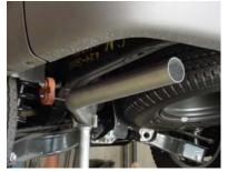
INSTALL EXIT PIPE # D AND INSERT WELDED HANGER INTO RUBBER GROMMET.
