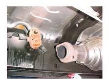
TO REMOVE STOCK EXHAUST UNBOLT IT FROM THE SLIP-FIT JOINT LOCATED IN THE REAR ABOVE THE AXLE AND SLIDE THE TAILPIPE OUT. NEXT UNBOLT THE 2-BOLT FLANGE LOCATED JUST BEHIND THE CATALYTIC CONVERTER. DO NOT THROW AWAY STOCK NUTS AND BOLTS YOU WILL NEED TO RE-USE THEM. LEAVE ALL RUBBER GEOMMETS ON THE HANGERS. USE WD-40 TO AID IN THE REMOVAL OF EXHAUST AND HANGERS.
