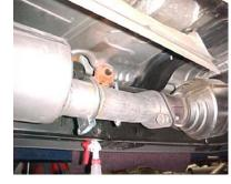
INSTALL HEADPIPE #A. SLIDE HEADPIPE INTO MUFFLER 1-1/2" TO 2" USE CLAMP # F TO SECURE HEADPIPE TO MUFFLER. DO NOT TIGHTEN. NEXT USE YOUR STOCK NUTS AND BOLTS TO SECURE HEADPIPE TO STOCK FLANGE.
