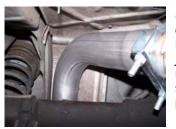
6. Install muffler assembly #B onto head pipe. Insert hangers into rubber grommets. Use a jack stand to support the muffler. Use clamp #G to secure the muffler to the head pipe. Do not tighten.
