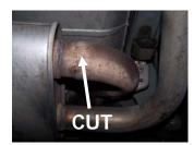
2. To remove the stock exhaust, cut off your stock over axle tailpipe just at the muffler. Then remove hangers from rubber grommets and remove muffler assembly.
