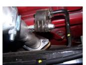
2. Install head pipe #A onto your existing stock flange using bolt kit #H to secure to flange. DO NOT TIGHTEN. Insert welded hanger into rubber grommet.
