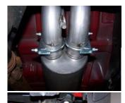
6. Install passenger side overaxle pipe #E into muffler 11/2 -2", secure using clamp #G. DO NOT TIGHTEN. Insert welded hanger into rubber grommet.
