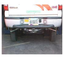
INSTALL EXIT PIPES #E ONTO TAILPIPES AND ATTACH TO HANGER #H AND CLAMP #G TO SECURE EXIT PIPES TO TAILPIPES. THESE METAL HANGERS NEED TO BE ROTATED IN ORDER TO ADJUST FOR CLAMPING. CUT TO YOUR PREFERED LENGTH. NOW INSTALL YOUR STAINLESS STEEL TIPS TO YOUR DESIRED LOOK. NOW YOU CAN TIGHTEN ALL CLAMPS, NUTS, AND BOLTS. STARTING FROM THE FRONT WORKING BACK. USE ZIP TIES TO TIE AWAY BRAKE LINES.
