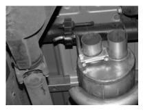
INSTALL MUFFLER #B ONTO HEADPIPE AT LEAST 1  $\frac{1}{2}$ " TO 2". USE CLAMP #F TO SECURE MUFFLER TO HEADPIPE. DO NOT TIGHTEN. USE A JACK STAND TO SUPPORT THE MUFFLER. OUTLETS SHOULD BE AT THE TOP.
