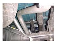
Install passenger side overaxle tailpipe #D into muffler 1  $V_2$ " to 2". Secure to muffler with clamp #H. Do not tighten.
