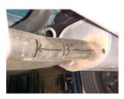
Lay out the exhaust on the floor so it looks like the drawing and compare parts with manual. **To remove the stock exhaust cut 13" just in front of the muffler.** Leave all rubber grommets in place. Use WD-40 to aid in removal of exhaust and hangers. Use hacksaw to cut tailpipe off.
