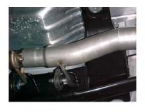
INSTALL HEADPIPE #A, YOU WILL NEED TO LINE UP THE TWO NOTCHES. INSERT WELDED HANGER INTO RUBBER GROMMET. USE CLAMP #A TO SECURE HEADPIPE TO THE STOCK PIPE. DO NOT TIGHTEN.
