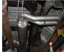
INSTALL MUFFLER ASSEMBLY #B ONTO HEADPIPE 1-1/2" TO 2". SLIDE WELDED HANGERS INTO RUBBER GROMMETS YOU MAY NEED TO ADJUST WELDED HANGERS TO FIT INTO YOUR GROMMETS. USE A JACKSTAND TO SUPPORT YOUR MUFFLER. USE CLAMP #C TO SECURE IT TO YOUR HEADPIPE. DO NOT TIGHTEN.
