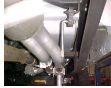
SLIDE DRIVERS SIDE TAILPIPE #D INTO MUFFLER 1-1/2" TO 2". INSERT WELDED HANGER INTO RUBBER GROMMET AND ATTACH TO MUFFLER USING CLAMP #H. THE PASSENGER SIDE TAILPIPE WILL BE ON THE BOTTOM.
