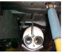
SLIDE PASSENGER SIDE TAILPIPE #E INTO OUTLET OF MUFFLER 1-1/2" TO 2". USE CLAMP #I TO SECURE TAILPIPE TO MUFFLER. DO NOT TIGHTEN.
