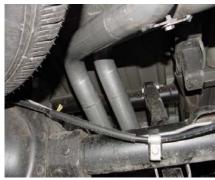
"MAKE SURE YOU HAVE A MINIMUM OF 1" CLEARANCE ON ALL PIPES FROM BRAKE AND FUEL LINES, TIRES, SHOCKS, ETC..."
