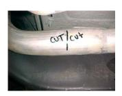
TO INSTALL YOUR GIBSON DOWN PIPE YOU NEED TO REMOVE YOUR STOCK EXHAUST. REMOVE IT FROM THE 4 BOLT FLANGE IN FRONT OF YOUR STOCK MUFFLER, CUT OFF YOUR STOCK TAILPIPE FOR EASIER REMOVAL. LEAVE ALL RUBBER GROMMETS IN PLACE. USE WD-40 TO AID IN REMOVAL OF EXHAUST AND HANGER. AFTER YOUR STOCK EXHAUST IS REMOVED YOU NEED TO REMOVE THE CATALYTIC CONVERTER FROM THE 2-BOLT FLANGE.
