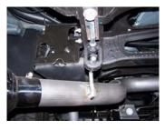
8. Install exit pipe #E onto the tailpipe 1.5-2" and secure with clamp #H. Do not tighten. Rotate pipe to best suit your vehicle. Insert welded hanger into rubber grommet. Adjust pipes to fit your vehicle with tips on so you make sure there is proper clearance.
