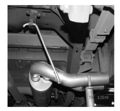
SLIDE MUFFLER ASSEMBLY ONTO HEADPIPE 1 1/2" TO 2". INSERT WELDED HANGER INTO RUBBER GROMMET ON DRIVERSIDE USE CLAMP #C TO SECURE MUFFLER TO HEADPIPE. DO NOT TIGHTEN.
