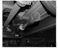
INSTALL HEADPIPE #B ONTO STOCK FLANGE, USE STOCK 15MM NUTS TO SECURE IT. DO NOT TIGHTEN, JUST MAKE SNUG.
