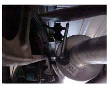
INSERT MUFFLER ASSEMBLY #A ONTO HEADPIPE AT LEAST 1-1/2" TO 2", USE A JACKSTAND TO SUPPORT MUFFLER ASSEMBLY. USE CLAMP #C TO SECURE MUFFLER ASSEMBLY TO THE HEADPIPE, DO NOT TIGHTEN. INSERT WELDED HANGER INTO RUBBER GROMMET.
